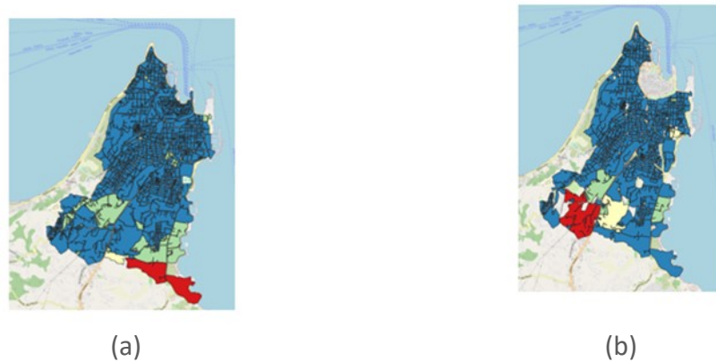
Figure 9: (a) Consequences for the water network in terms of percentage of people with access to water; (b) Consequences for the Tier 3 buildings in terms of percentage of buildings that collapsed.
