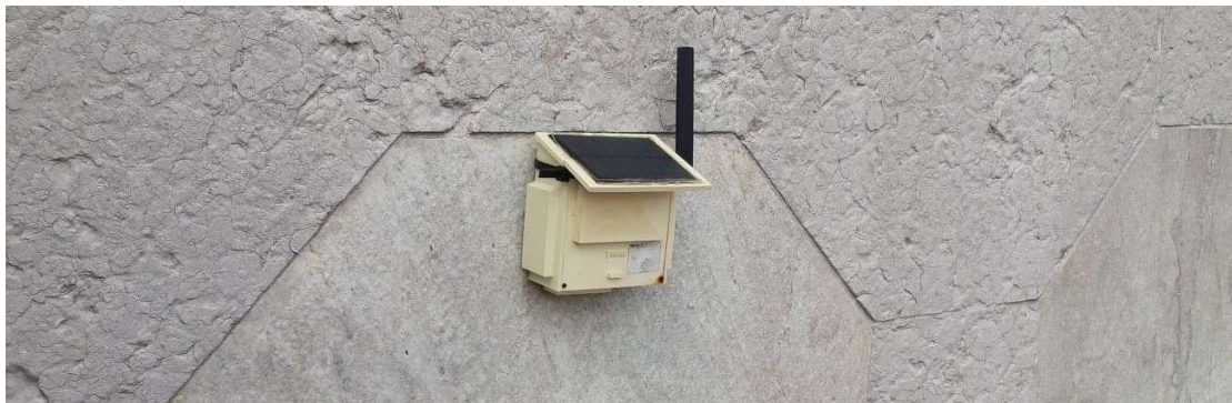
Figure 3: A HYPERION smart sensor tag place on the Torre dell' Orologio in Venice
