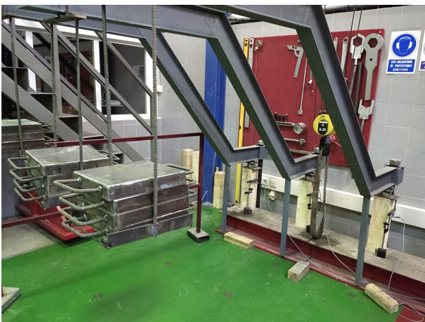
Fig. 3 Configuration of the creep tests
