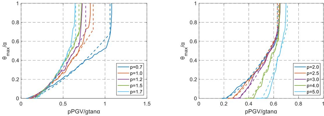
**Figure 6.** Median seismic demand estimates for rocking blocks with different characteristic parameters over a range of intensity levels. Results are presented for the dimensionless PGV. Fit is shown with dashed lines.
