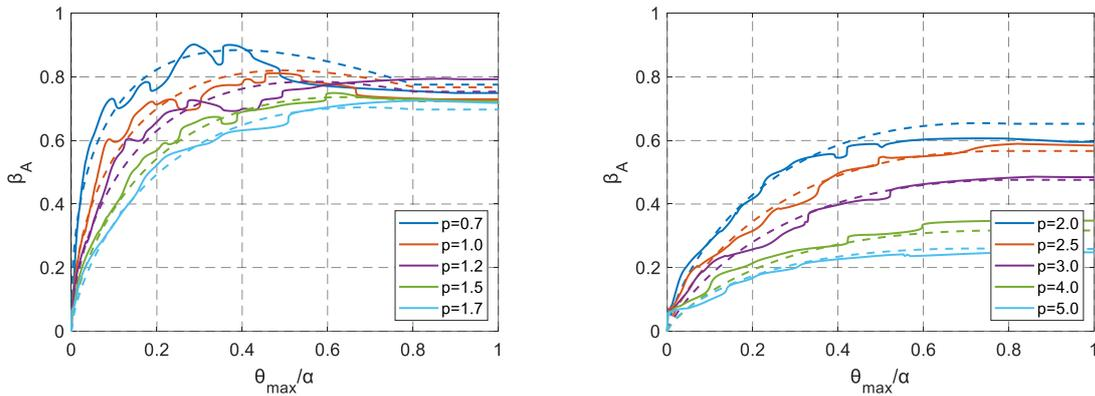
**Figure 5.** Dispersion estimates for rocking blocks with different characteristic parameters. Results are presented for the dimensionless PGA. Fit is shown with dashed lines.
