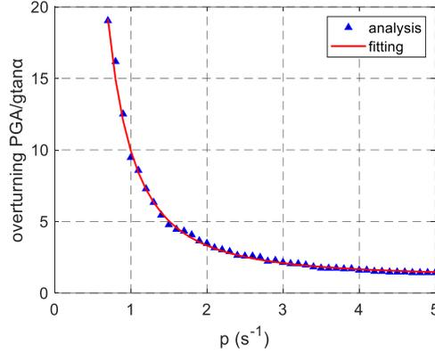
**Figure 4.** Median seismic demand for the first occurrence of overturning considering the dimensionless PGA as an IM.
