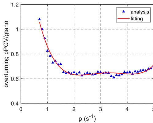
**Figure 7.** Median seismic demand for the first occurrence of overturning considering the dimensionless PGV as an IM.
