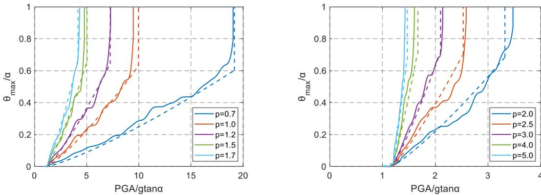
**Figure 3.** Median seismic demand estimates for rocking blocks with different characteristic parameters over a range of intensity levels. Results are presented for the dimensionless PGA. Fit is shown with dashed lines.
