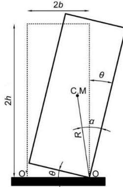
**Figure 1.** Rocking block geometry
