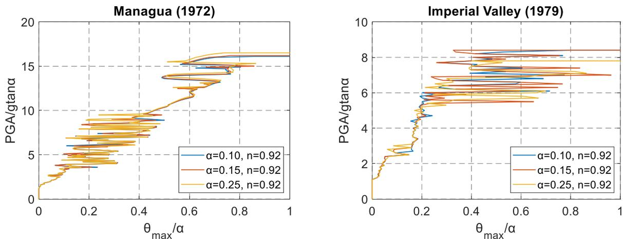
**Figure 2.** IDAs for two different earthquake records for variable block stability angles  $\alpha$  and a constant coefficient of restitution  $\eta$  considering a rigid block with  $p=1 \text{ s}^{-1}$ .
