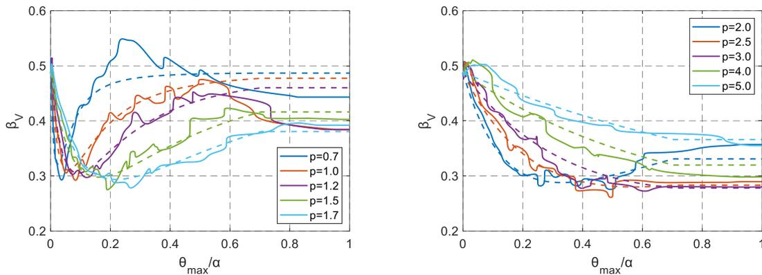
**Figure 8.** Dispersion estimates for rocking blocks with different characteristic parameters. Results are presented for the dimensionless PGV. Fit is shown with dashed lines.
