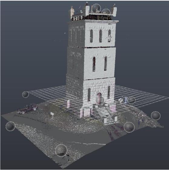
Fig. 2. Point clouds derived from the 3D laser scanner and position of the scanners
